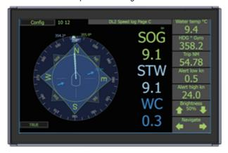
SKIPPER DL2 is a dual axis doppler speed log providing you Speed Through Water (STW) and Speed Over Ground (SOG) in two or three axis (Docking Mode). The resultant sea current will also be calculated in speed and direction.
